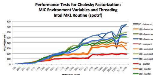
Figure 17: Cholesky Factorization (SPOTRF) Performance Test: Comparison of Different MIC configurations
