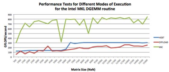
Figure 12: Intel MKL DGEMM Performance Test: Modes of Execution
