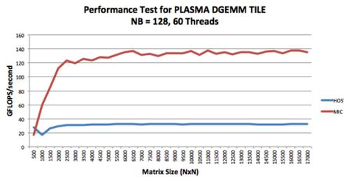
Figure 10: PLASMA Tiled DGEMM Performance Test
