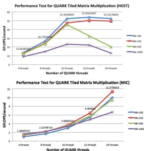
Figures 8 + 9: QUARK Performance Test for Host and MIC
