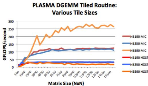
Figure 11: PLASMA Tiled DGEMM Test with Different Tile Sizes
