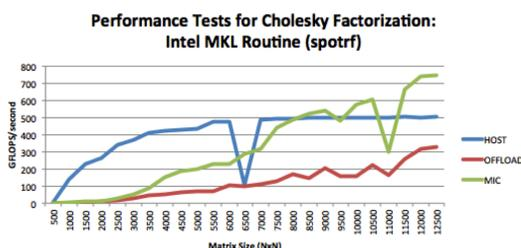
Figure 16: Cholesky Factorization (SPOTRF) Performance Test
