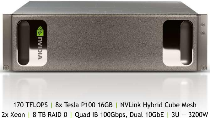
2x Xeon | 8 TB RAID 0 | Quad IB 100Gbps, Dual 10GbE | 3U - 3200W
