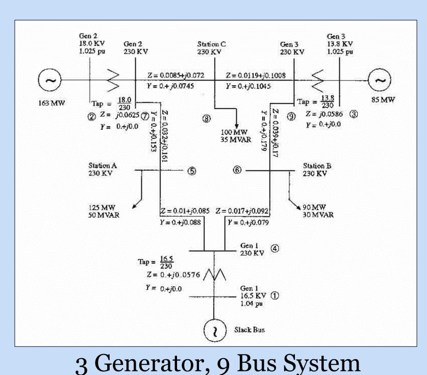
The MatPower program takes an admittance matrix created from a bus diagram as input and solves the power equations for the state variables.
