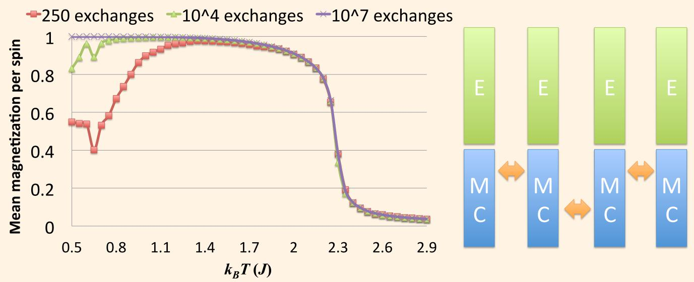
Replica exchange among random walkers at different temperatures lowers correlation, thus improves convergence. However, variance data (e.g. susceptibility) is not converging well. We suspect that some simulations are not fully equilibrated before MC sampling starts. When we allow replica exchange during equilibration, the improvement is instant.
