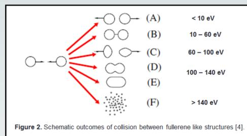
Figure 2. Schematic outcomes of collision between fullerene like structures [4].
