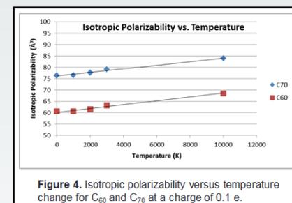
Figure 4. Isotropic polarizability versus temperature change for  $C_{60}$  and  $C_{70}$  at a charge of 0.1 e.
