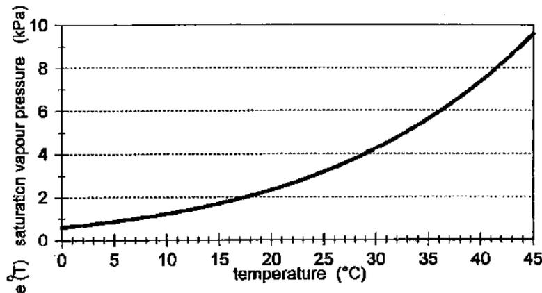
Figure 1 Saturation vapor pressure vs Temperature
