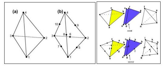
**Figure 6:** (a) Four node tetrahedral (b) Ten node tetrahedral **Figure 7:** Six node and twelve node interfaces
