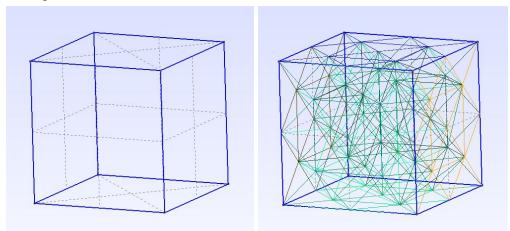
Figure 2: A simple cube created in Gmsh on the left. A three dimensional mesh of the cube on the right.
