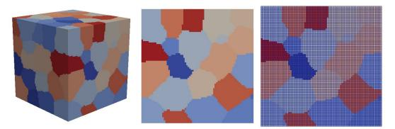
Figure 4: Microstructural grains created using Dream3D in the cube example from Figure 2.
