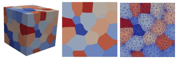
Figure 5: Dream3D grain structures modified by Voxel2Tet to have smoother interfaces.
