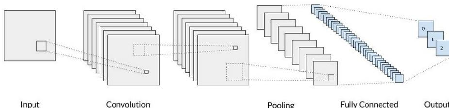
Figure 3: CNNI-BCC Architecture
