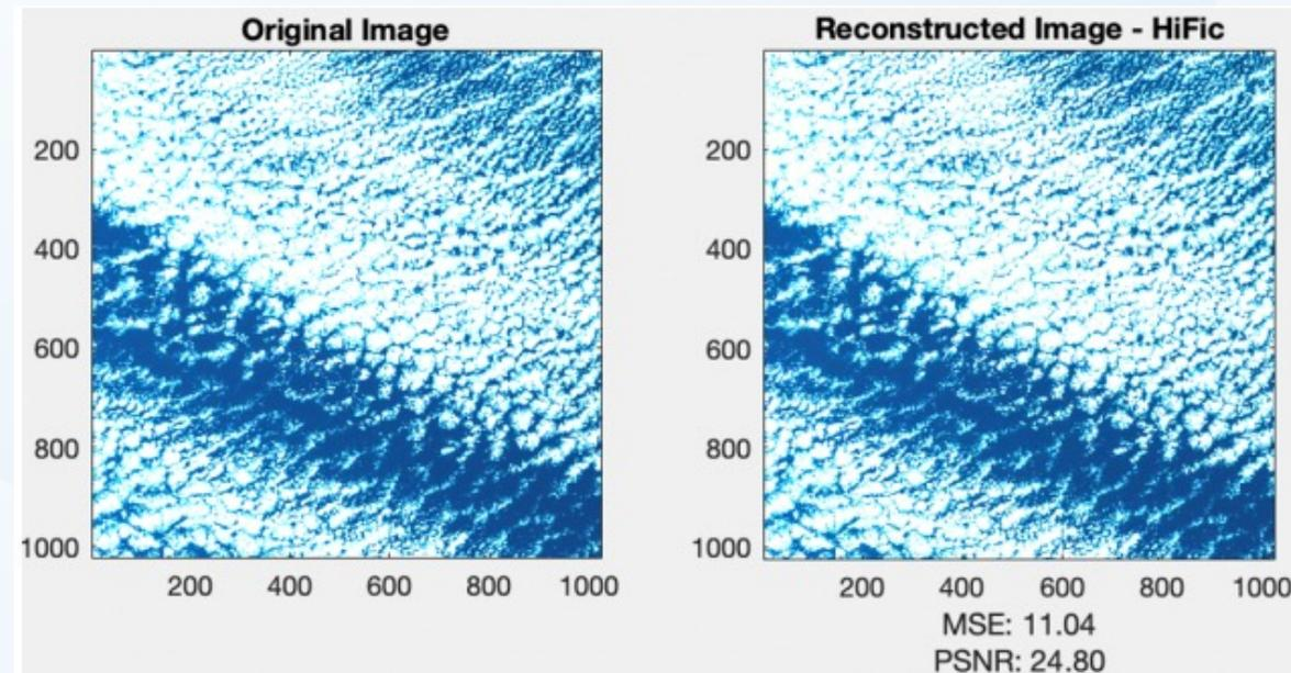
The reconstructed image's MSE and PSNR are only slightly worse than the wavelet compression while saving significantly more space. The reconstructed image shows virtually no visual difference from the original.
